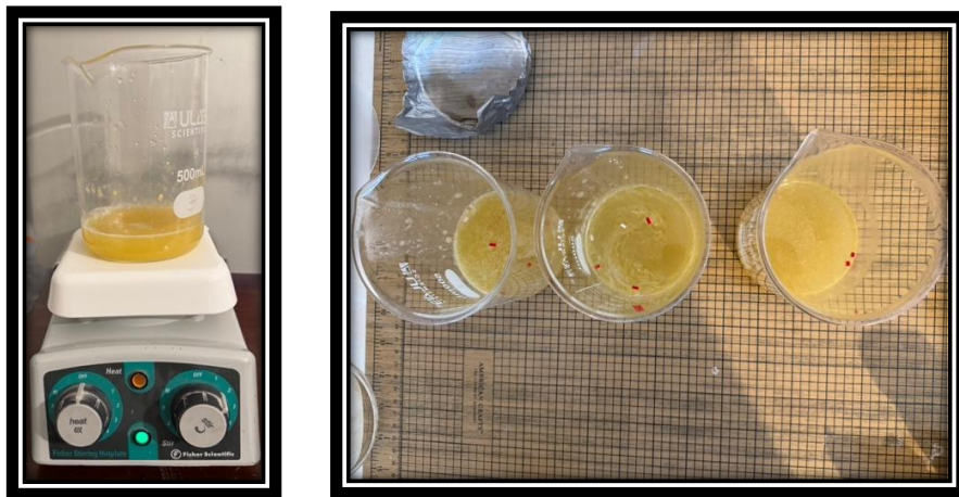
Figure 6: Stirring and density separation of microplastics in solid residuals (taken by Zenaida Rosa).
