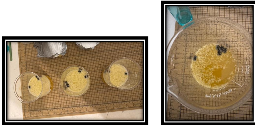
Figure 5: Samples after heating digestion and sprayed with 70% isopropyl alcohol (taken by Zenaida Rosa).
