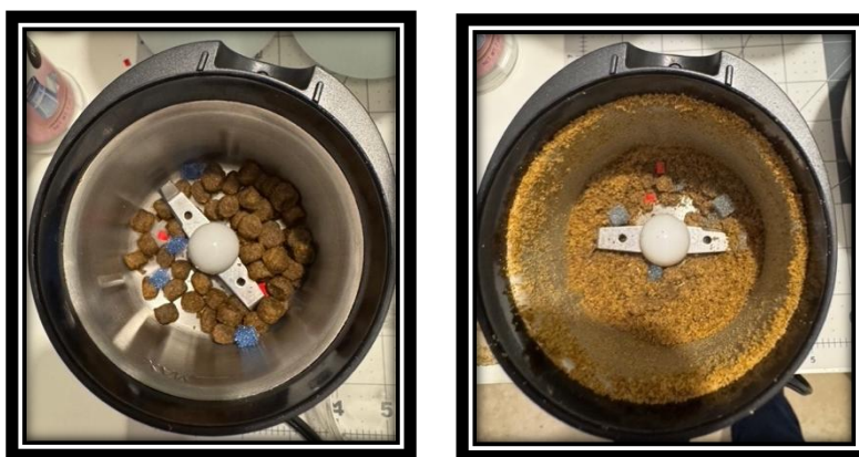
Figure 9: Testing the homogenization of dog feed with an electric grinder (taken by Zenaida Rosa).
