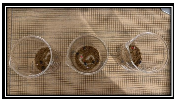
Figure 3: Homogenized dog feed samples spiked with plastics (taken by Zenaida Rosa)
